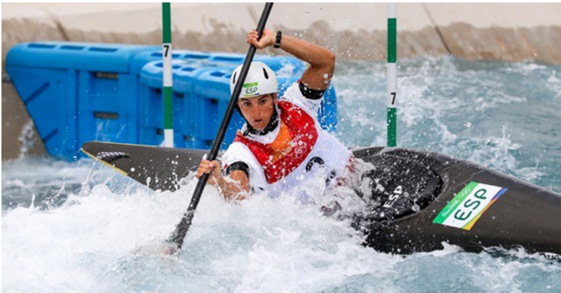
Figure 2.25 Maialen Chourraut (representing Spain) on her gold medal-winning run at the Rio 2016 Olympics. Note the high-volume front deck area and the low-volume rear deck. The helmet is a lightweight plastic model, and there is a sport-specific low-volume buoyancy aid. The tight-fitting neoprene spraydeck ensures virtually no water enters the boat. The paddle as well as canoe are constructed of carbon fiber. Source: Balint Vekassy, © ICF.
